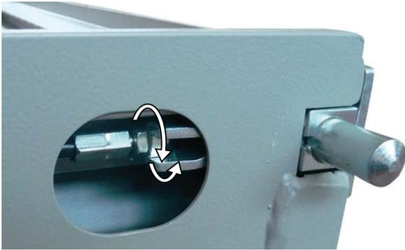
**1** Loosen the locknut using an appropriate wrench.
