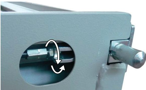
**3** Once the cable is adjusted correctly, and the levers are functioning properly, Tighten the lock nuts.
